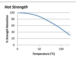
"Hot strength" shear strength. Fully cured specimens conditioned to pull temperature for 30 minutes before testing at temperature.
