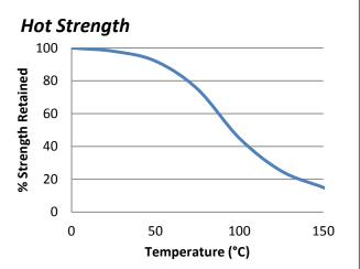
"Hot strength" shear strength tests performed on glass to mild steel. Fully cured specimens conditioned to pull temperature for 30 minutes before testing at temperature.
