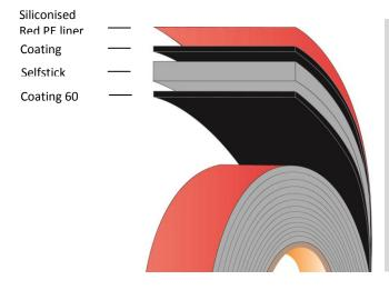
Thickness: 0,64mm (0.025 inch)  $\pm$  15% Core: Conformable acrylic Adhesive: Acrylic coating 60 Density:  $600 \text{kg/m}^3 (37 \text{lb/ft}^3)$
