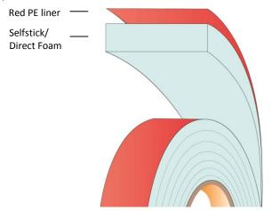
Thickness: 1,0 mm  $(0.039 \text{ inch}) \pm 10\%$ Core: Closed cell acrylic
